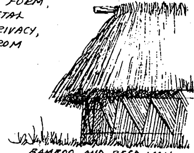
BAMBOO AND REED WALL FIJI ISLANDS
