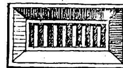
STONE VENTILATION GRILLE GUANAJUATO, MEXICO
