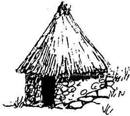
TEMPORARY MOUNTAIN SHELTER, PAKISTAN - EARTH AND ROCKS ARE PILED UP AROUND PART OF THE STRUCTURE.
